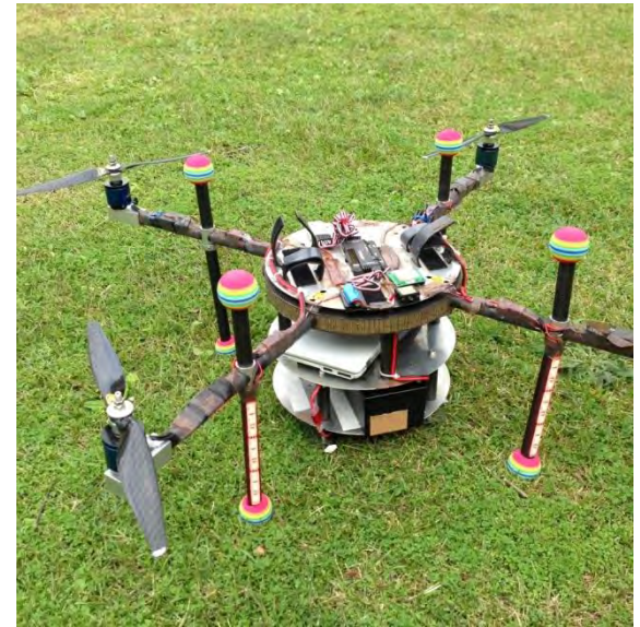
Quad copter Four rotors Payload 5kg
