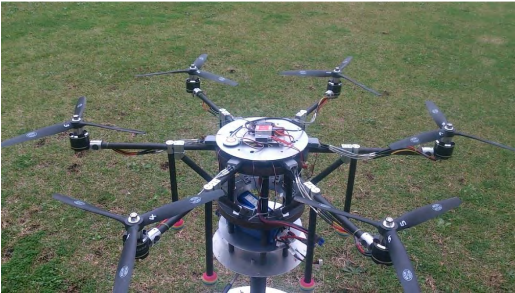
Hexa copter Six rotors Payload over 20kg
